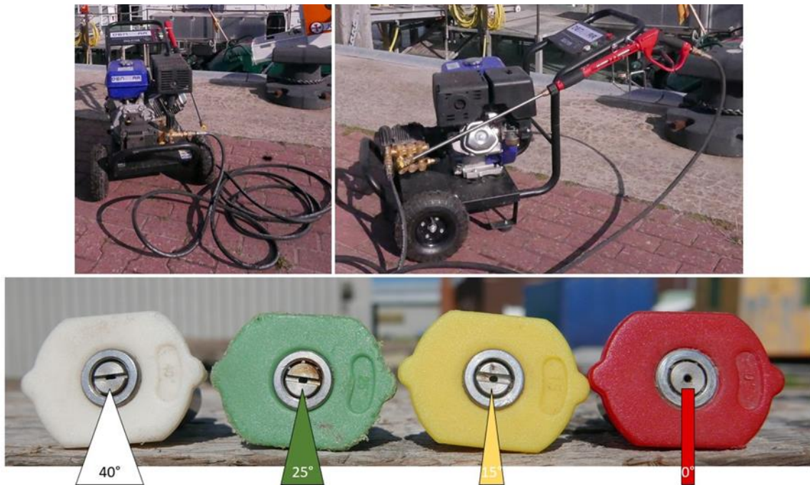
Fig.17: Top: Petrol-powered high-pressure washer; bottom: Nozzles and the corresponding angles of the exiting water jet
