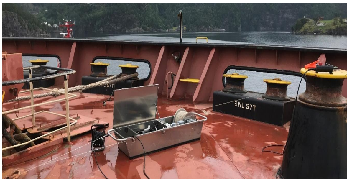
Fig.1: Winch on forecandle deck with rope via fairlead
