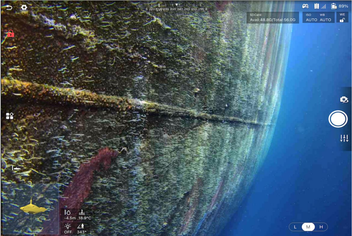
Fig.5: Indicative of the Heavy Slime condition, typical in the current traditional ‘scrub mentality’ - addressing underwater hull maintenance, with a ‘too fouled to operate’ approach.
