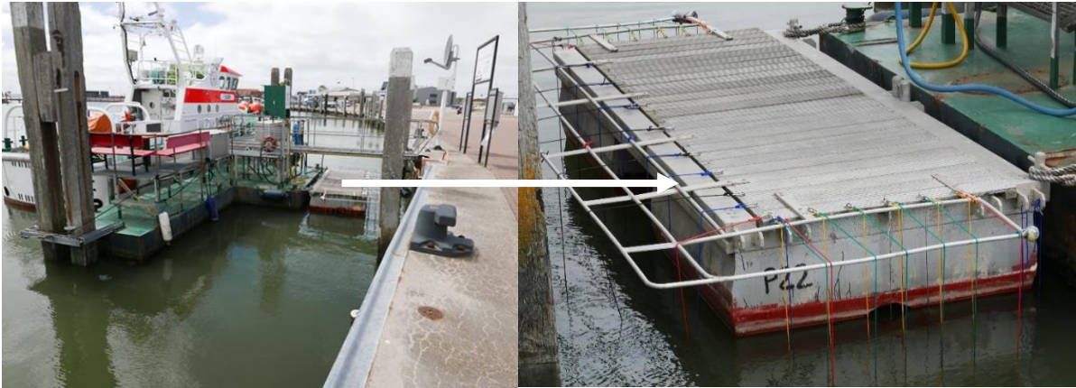
Fig.12: One pontoon for static exposure of test panels in the harbour Norderney
