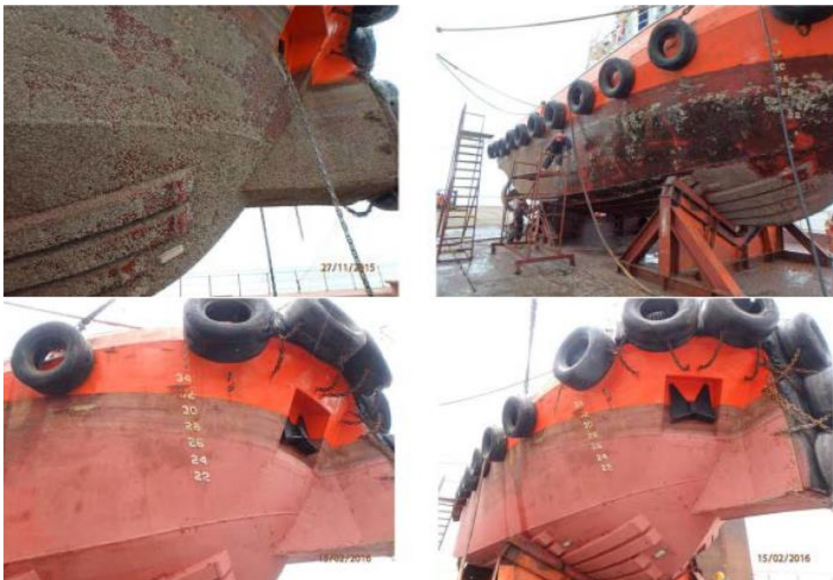
Fig.8: Tugboat without (top) and with (bottom) ultrasonic antifouling protection
