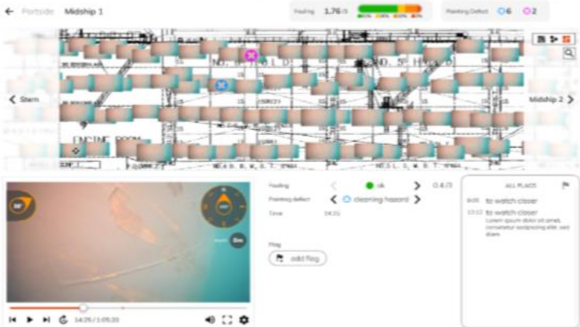
Fig.3: Inspection with localized images placed on the general arrangement plan of a vessel
